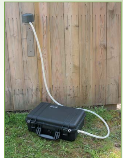
DPS System in use. DPS Impactor shown with rain cap.
